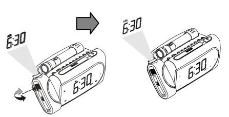
6.) If you no longer wish to see the projected image, press the **PROJECTOR** 'On/Off' button to turn the projector 'Off'.
